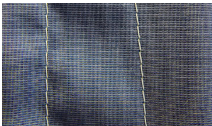
Fig. 5: Left seam: sewn in warp direction Right seam: sewn at 2° bias to warp direction.
